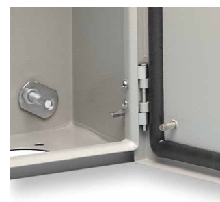
The enclosure has welded M8 bolts in the bottom of the base and M6 bolts in the door. There is also an M6 bolt for earthing on one side.
