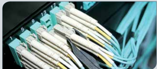
Jaw retains connector allowing it to be pulled free
