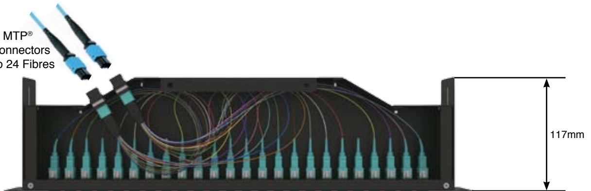
2 MTP® connectors to 24 Fibres
